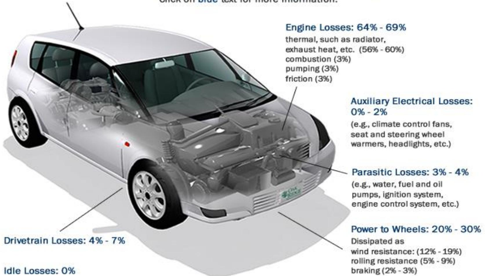
In this figure, they are accounted for as part of the engine and parasitic losses.
